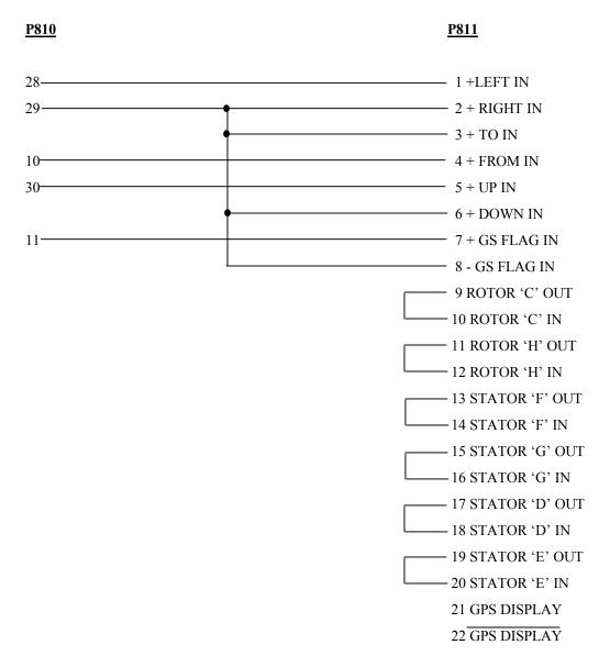
FIGURE 2-2 ADDITIONAL BENCH TEST HARNESS FOR NAV122D/GPS
