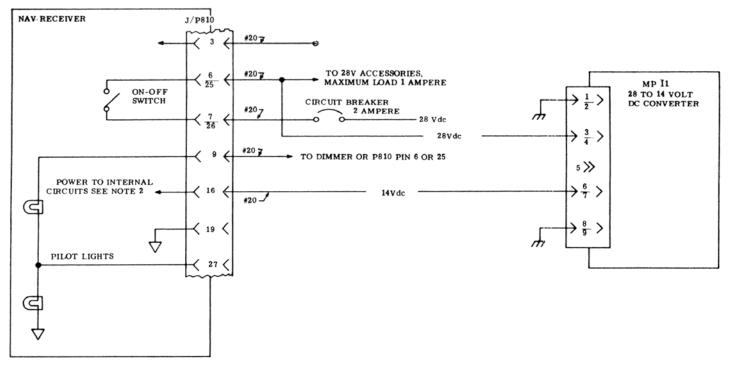
FIGURE 2-8 POWER INPUT CONNECTIONS
