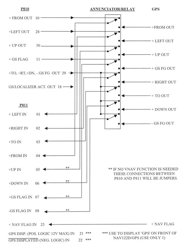
**Figure 2-10A**NAV122D/GPS, IFR GPS, and GPS annunciator relay diagram
