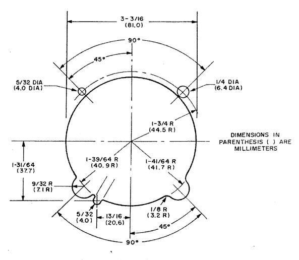
FIGURE 2-4. MOUNTING TEMPLATE, REAR MOUNT (Not drawn to size, for reference only)
