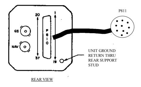
FIGURE 2-6. BNC CABLE CONNECTOR
