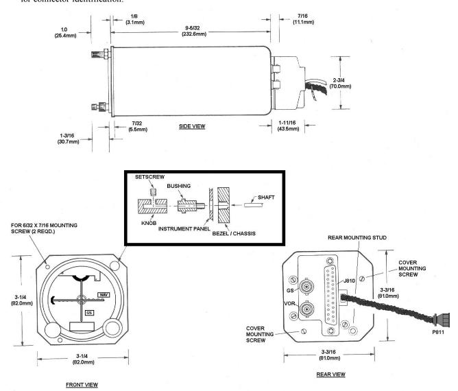
FIGURE 2-3. MECHANICAL INSTALLATION
