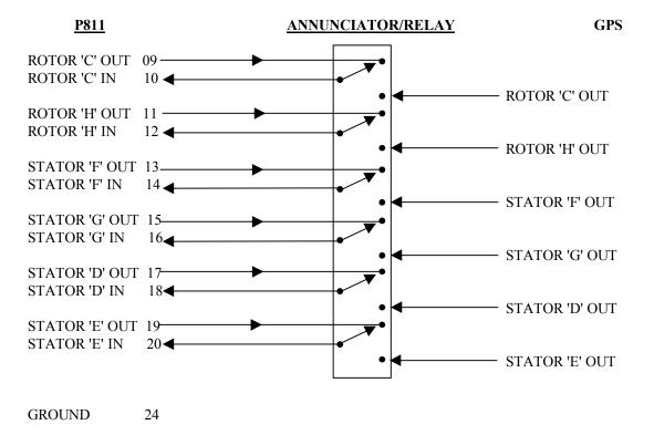
Figure 2-10B NAV122D/GPS, IFR GPS, and GPS annunciator relay diagram
