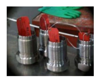
Terminals, Poured Type 1-7/16" Diameter Cable p/n 421404-1 Rev L
