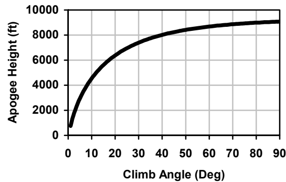
Figure 12 Variation of Apogee Height with Climb Angle
