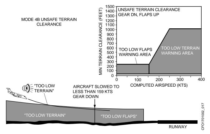
**NOTE:** Aural "TOO LOW FLAPS" warning can be silenced by selecting OFF on the FLAPS switch, which is located on the TAWS WARN panel.
