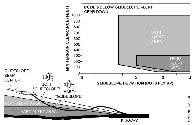
**NOTE:** The "GLIDESLOPE" aural warning can be muted by selecting the GS switch OFF, which is located on the TAWS WARN panel.
