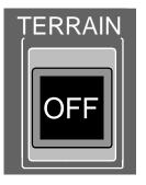
**NOTE:** When landing at an airport that is not in the database, TERRAIN functions can be inhibited by selecting the TERRAIN switch OFF. The switch is located on the TAWS WARN panel.
