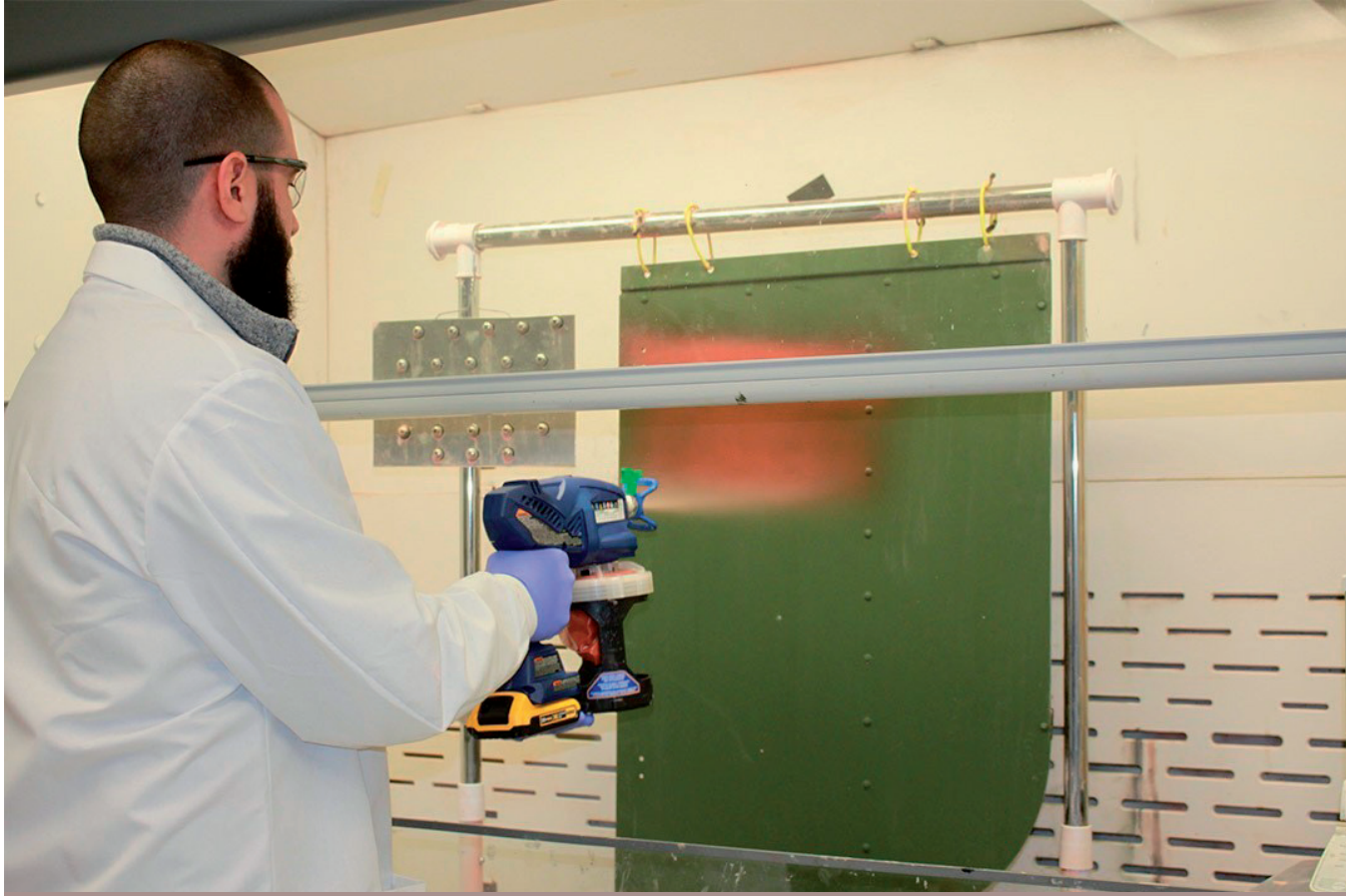
Clear Scientific Senior Scientist Patrick Reust applies Decon Slurry to a vertical surface in the company's research laboratory.
