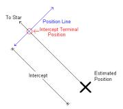
The observed distance is known as the **True Zenith Distance** (TZD.) The value based on the assumed position is the **Calculated Zenith Distance** (CZD.) The difference between the two is known as the **Intercept**.
