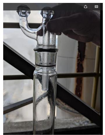
Picture 1 - Dropout Impinger
