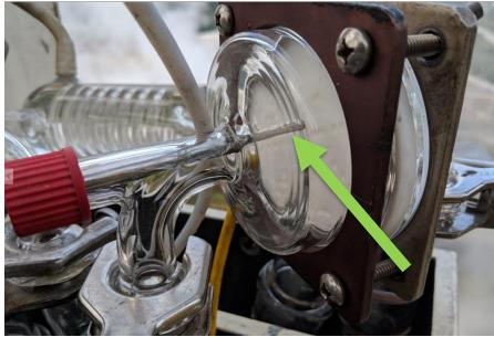
Picture 4 – CPM Thermocouple
