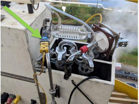
Picture 6 – Exit Impinger Thermocouple
