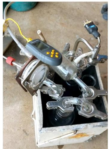
Picture 8 (Nitrogen Purge Setup – white line is N<sub>2</sub> gas coming from UHP nitrogen tank (green at top); temperature sensor pictured (device with yellow buttons)
