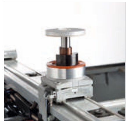
Hyperclamp for rigid and precise locking.
