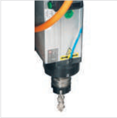
Fixed vertical motor dedicated to additional milling operations (slot, anti-splintering, etc.).
