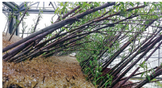
In NCHRP Project 24-39, researchers grew willow trees to maturity in a greenhouse to test how well they protect embankments from scour.
