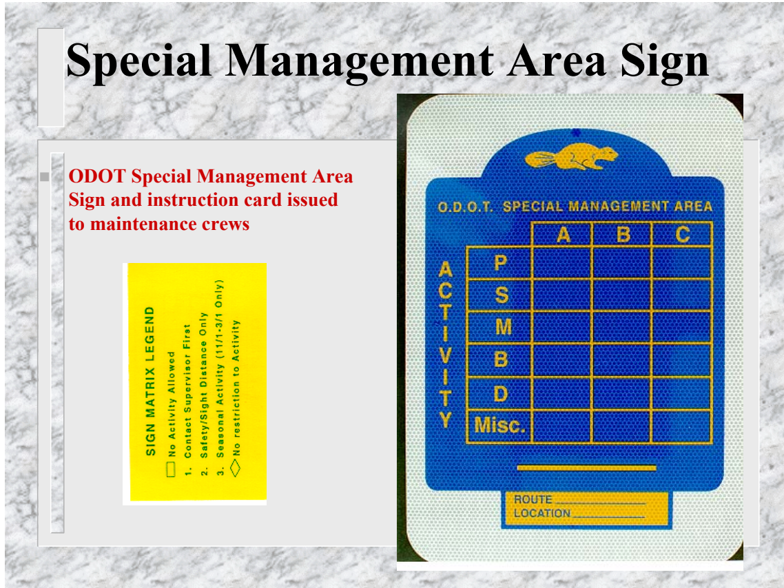
Figure 16: ODOT Special Management Area Maintenance Sign
