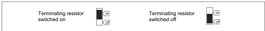
Figure 7-10 Terminating resistor switched on and off
