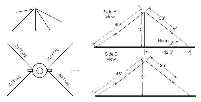
The EZ NVIS is ready to deploy NVIS antenna based on an article by Carl Jelnick, N6VNG (SK). He based his design on the AS-2259/GR a military, dual band NVIS antenna set. The antenna comes with a center support and the four assembled and marked antenna elements. You need to add rope, coax and an appropriate mast. The antenna is constructed from 14ga Soft Drawn copper wire.
