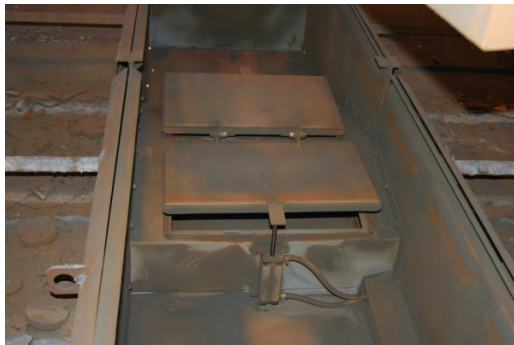
Fig. 1. Section of a cutting table with damper doors.
