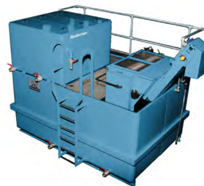
Fig. 5. The Perpetum system connects to several machines, continuously removing bacteria. This system reduces the number of necessary coolant changes by more than 90 %.
