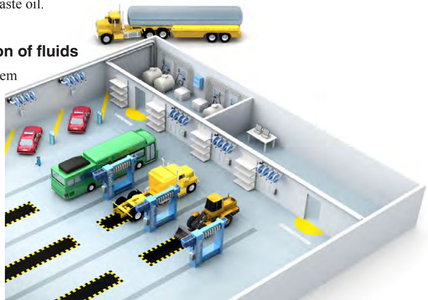
Fig. 1. The centralized storage and distribution system simplifies the distribution of fluids in a vehicle repair shop.
