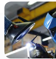
Welding fume extraction
