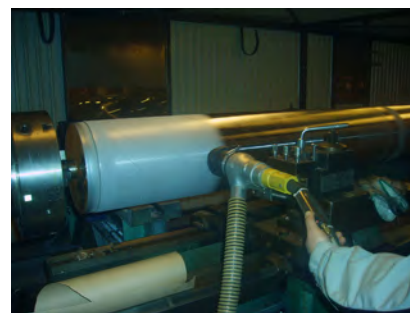
Fig. 4. On-tool vacuum blaster mounted on a lathe.
