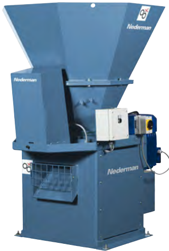
Fig. 2. Swarf Handling and Processing The integrated system crushes the swarf, de-oils the chips and recovers coolant.
