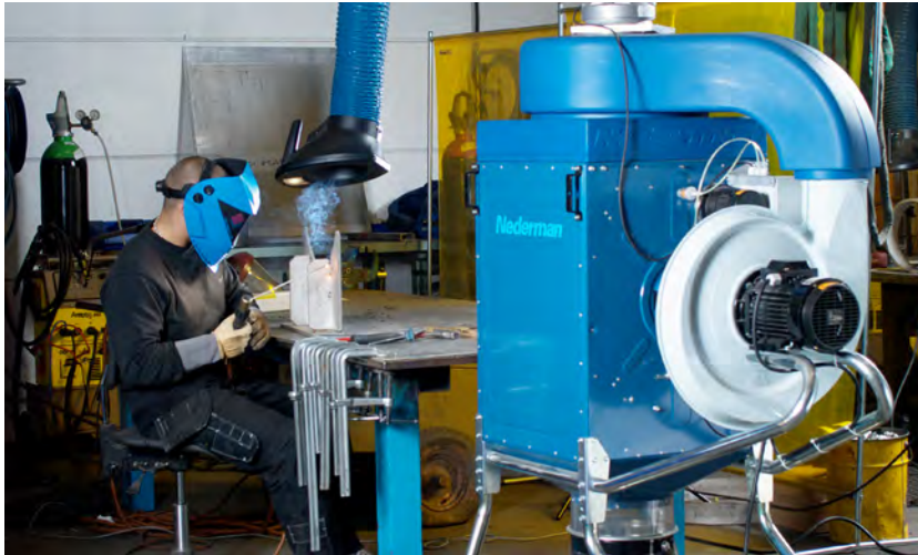
Fig 1. Proper positioning of extraction arm.
