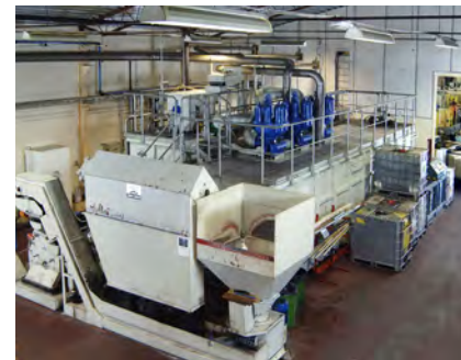
Fig. 2. Coolant Filtration Systems Our coolant cleaning solutions cover most operational requirements. This includes the Presto System that delivers coolant to two or more machine tools of the same type.
