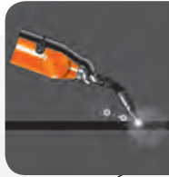
Robotic welding fume extraction
