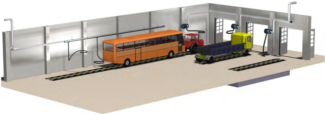
Fig. 1. A vehicle exhaust extraction installation with exhaust hose reels and fan.
