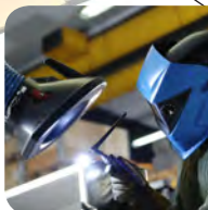
Extraction arms for welding fumes
