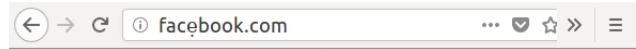
Figure 1: An example of the internationalized domain name xn--facebook-ts4c.com (homograph), which is displayed as facebook.com in the address bar.
