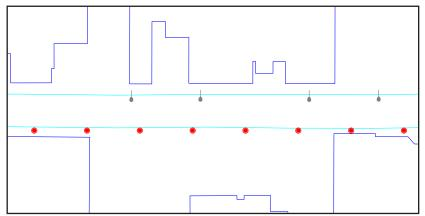
Not to scale plan view - alternate layout: pedestrian poles evenly spaced on one side of street only
