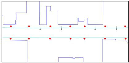
Not to scale plan view - alternate layout: pedestrian poles spaced between cobra-head streetlights
