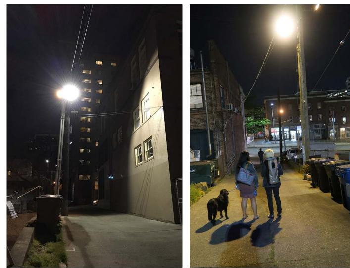
New LED floodlight - cool CCT, poor CRI, and more glare from multi-cell source
