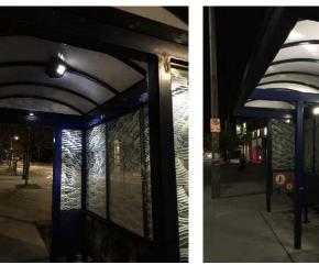
Internal lights are of various types, some lighting the roof, others lighting glass patterns - all are direct view and have significant glare.
