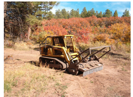
Figure 4. Mechanical treatment using a timberaxe.
