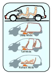
Figure 10 – Honda Fit fuel tank location and seating modes
