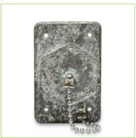
Images shown after parts subjected to 200 hour salt spray test
