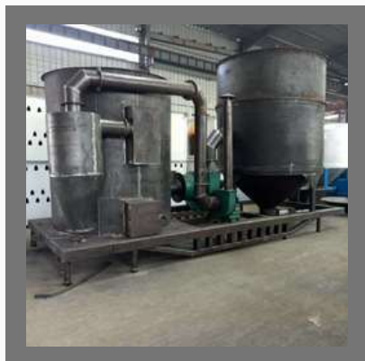
Diesel Fired Dryer
