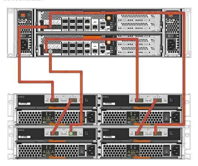
You have just cabled a new shelf to a FAS8200. Running the system node run -node \* sysconfig - a command indicates that multipath HA is configured. However, after running Config Advisor, you receive an error that your cabling is incorrect.
