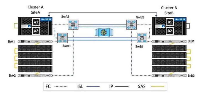
You are investigating an AutoSupport Disk Redundancy Failed alert. Cluster A lost connectivity to storage bridge BrB1, while cluster B lost connectivity to storage bridge BrA1.
