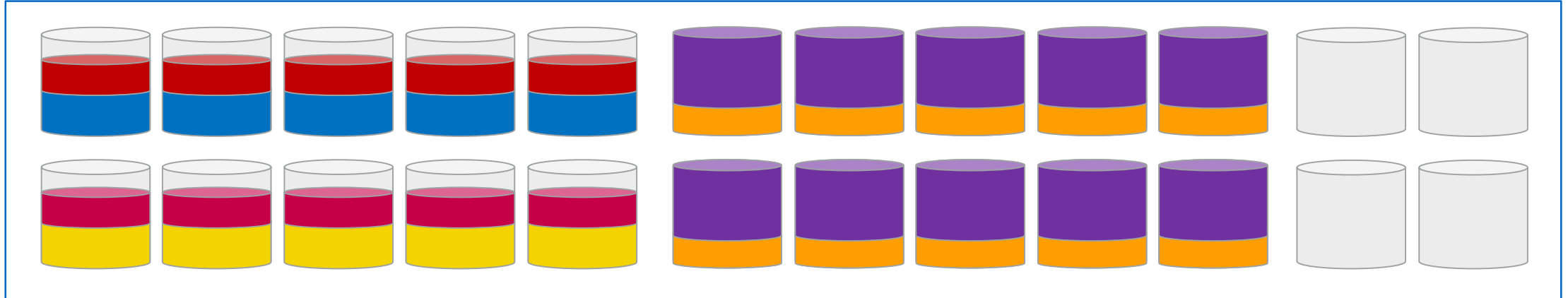
24-drive system with 2 10-drive groups (8+2) and 4 hot spares
