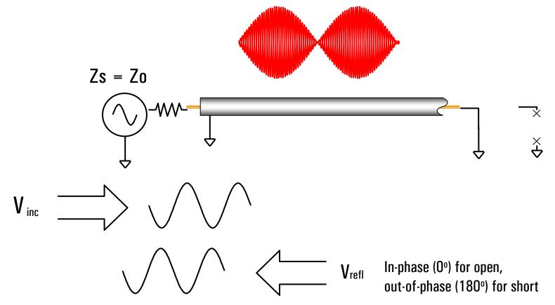
For reflection, a transmission line terminated in a short or open reflects all power back to source
