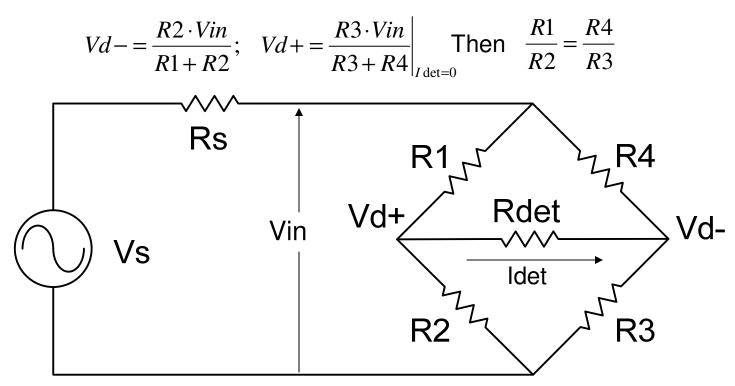
Further, it can be shown, that the input impedance of a balanced bridge follows the equation:  $Zin^2 = R1 \cdot R3 = R2 \cdot R4$
