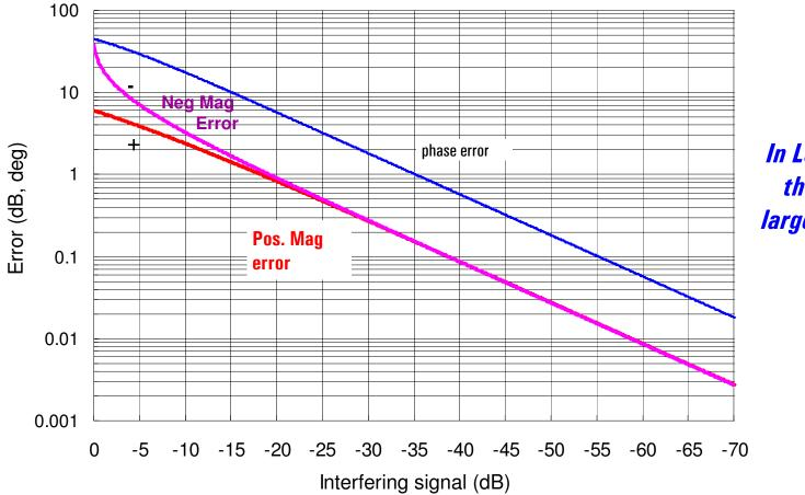
In Log Mag format, the -dB error is larger than the +dB error
