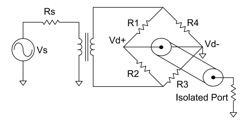
We would like the bridge to be matched so Rs<sup>2</sup>=R1\*R3=R2\*R4. In this condition, Vin=Vs/2.
