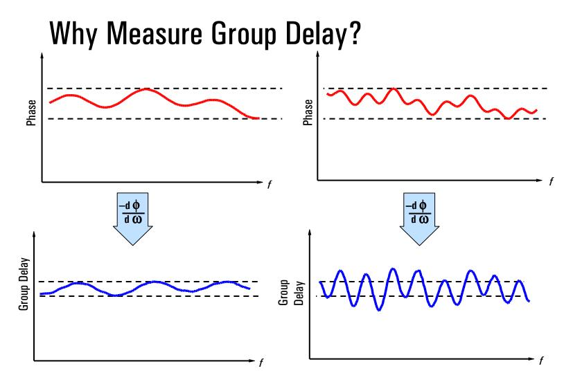
Same p-p phase ripple can result in different group delay
