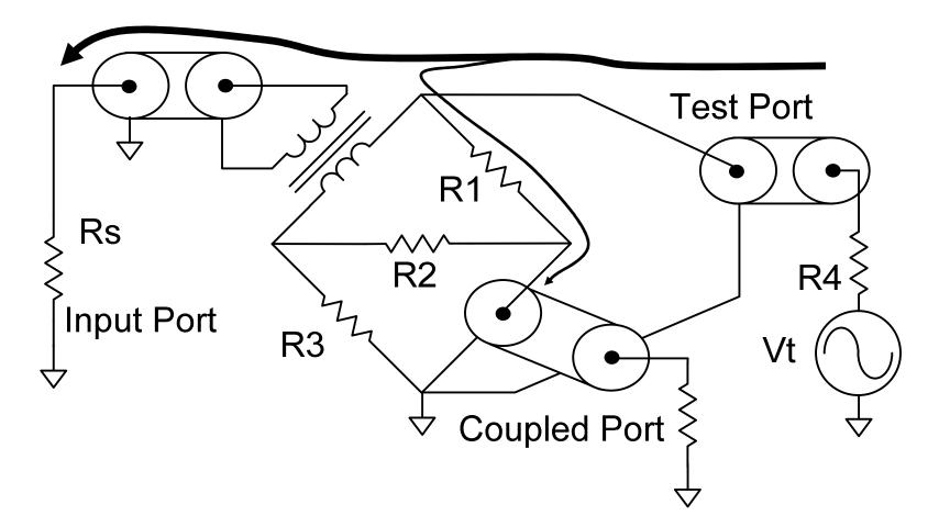
Let's check two cases: Assume the test port is open circuit (R4 infinite), then the voltage at the isolated point will be  $(1/2)^{*}(5/6)^{*}(1/6)^{*}Vs$ , exactly the same as the combination of loss and coupling, assuming a total reflection at the test port.
