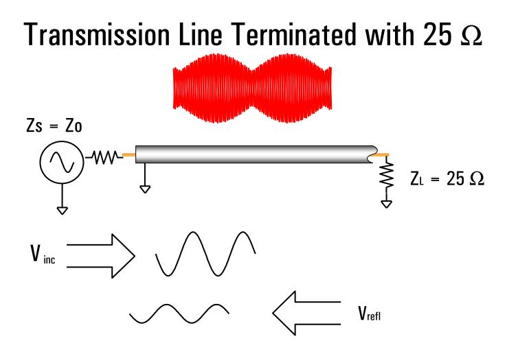
Standing wave pattern does not go to zero as with short or open
