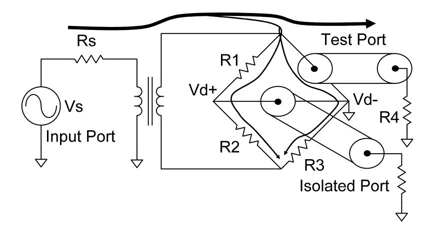
Now we can set the forward loss of the bridge. The voltage on the test port is equal to the voltage across R1. We have complete flexibility to set any ratio we want. In this case let's choose the voltage to be 5/6 of Vin. Then  $Vd_{+}=Vd_{-}=(1/6)Vin$ . The loss from Input Port to output port is  $20*\log(5/6) = -1.58$  dB.
