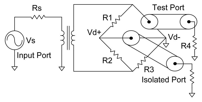
So, in the isolation direction it is clear that no signal appears at the isolated port, as the current divides equally across the bridge, if the test port is terminated in Rs
