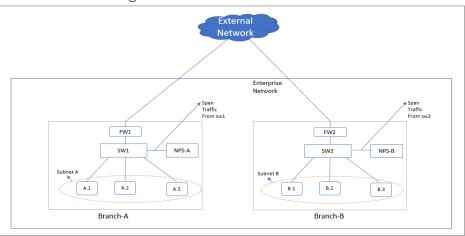
The enterprise network in the above scenario has 2 branches A and B. There are 2 sensors deployed one each in branch A and B. For the enterprise network subnets A and B together make up the range on IPs for internal assets that have to be inventoried. Assets A.1, A.2, and A.3 belong to subnet A and B.1, B.2, and B.3 belong to subnet B.
