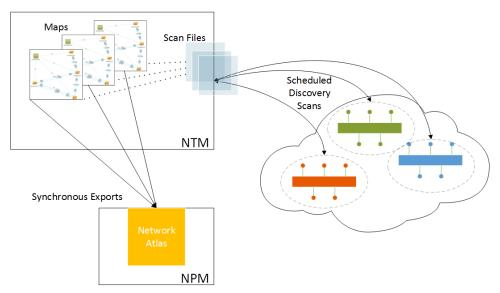
NTM's topological overview complements your primary network monitoring system (SolarWinds Network Performance Monitor (NPM), powerfully enhancing event triage by quickly showing how an issue with a particular node impacts larger aspects your network. While NPM lists alerts in order or urgency, NTM by distributing alerts on a map that clearly indicates, for example, that a particular switch sits in the path of all other alerting nodes.
