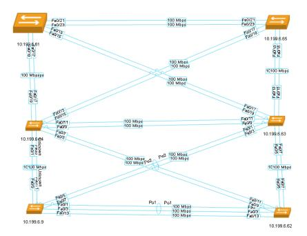
The **Link Speed** options only affect the displayed coloring of layer 2 links by speed range, and the display of **Speed by text**. When link speed is cleared, all connections show as grey lines.
