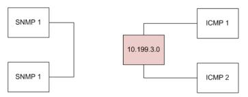
Node 10.199.3.0 is a Network Segment node that indicates the subnet in which the two discovered ICMP nodes are connected.
