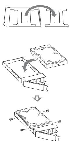
Fully insert the tray in which the HDD is installed into the slot, and lock it into place.
