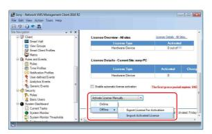
**5** Select the activated software license file stored on the USB flash memory device in the file opening screen, and click [Open].
