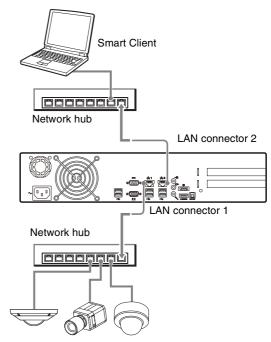
Network cameras Connect LAN connector 1 to the same network as the network cameras.
