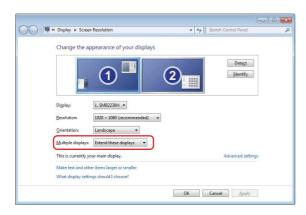
**3** Drag the displays under [Change the appearance of your displays], and match the positions of displays 1 and 2 with the actual positions of the monitors.
