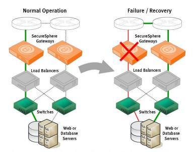
Diagram of Active-Passive Failover in a Redundant Architecture
