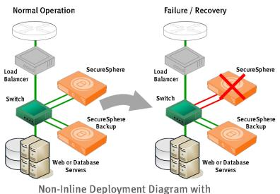
Non-Inline Deployment Diagram with Redundant SecureSphere Gateways
