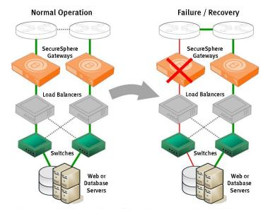
Diagram of Active-Active Failover in a Redundant Architecture
