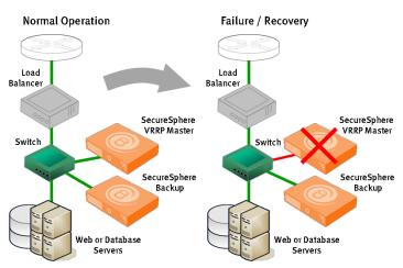
Diagram of Active-Passive Failover in Proxy Mode
