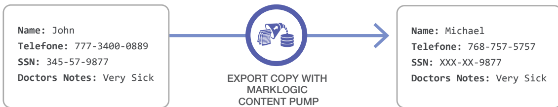
Figure 5: Redaction is similar to element level security, but is designed to control who sees what data when the data is exported from MarkLogic.
