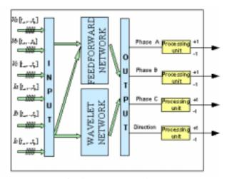
Fig. 4. MLF-DWT relay
