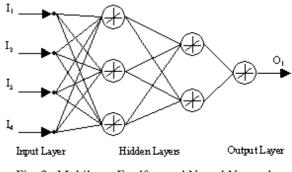
Fig. 3. Multilayer Feedforward Neural Network
