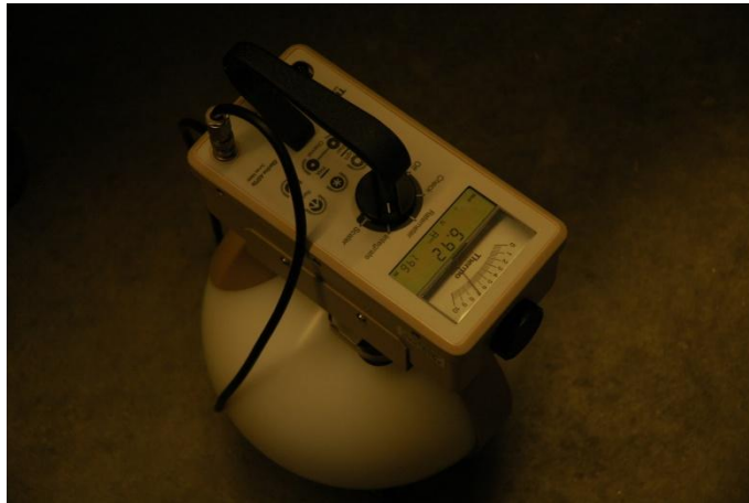
Figure 39: Neutron Detector registering Neutron Flux
