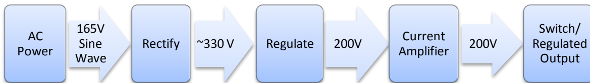
Figure 17: High Level View of Grid Power Supply
