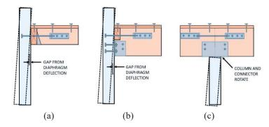
Figure 4. Wood framed, wood sheathed diaphragm connections (a) joist to perimeter concrete or masonry wall, (b) girder connection to perimeter concrete or masonry wall, and (c) girder to interior column.
