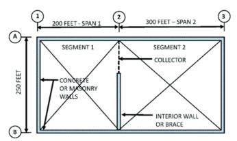
Figure 1b. Structure in plan view, divided into rectangular diaphragm segments for purposes of transverse seismic design. The Line 2 collector serves as a boundary between diaphragm segments for transverse direction loading.
