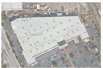
Figure 2. Structure with non-rectangular diaphragm is beyond the scope of these provisions.
