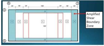
Figure 3. Diaphragm plan view with the amplified shear boundary zone indicated by shading.
