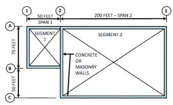
Figure 1a. Structure in plan view, divided into rectangular diaphragm segments for purposes of transverse seismic design. Note that identification of different segments will be required for longitudinal diaphragm forces.
