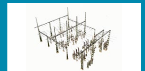
Figure 2: Example of a scan of a high voltage switch station
