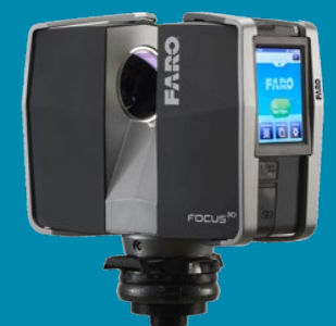
Figure 1: Faro focus 3D laser scanner
