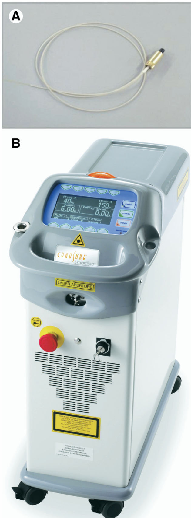
Figure 7 Laser-assisted liposuction device. SmartLipo fiberoptic handpiece and power source. (Courtesy of Cynosure.) (Color version of figure is available online.)
