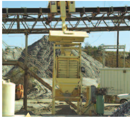
An automated sample dryer and gradation device can be integrated with a belt sampler to provide data on aggregate consistency.
