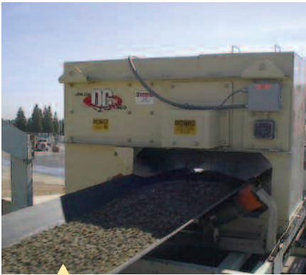
An automated belt sampling device can be used to sample the aggregate before it enters the dryer.
