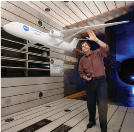
Wind-tunnel testing of subscale models of possible future aircraft configurations is still a vital tool in the R&D process. (left to right) A model of the transonic truss-braced wing design, a model of the D8 “double bubble” ultra-efficient subsonic design, and a model of a quiet supersonic technology design.
