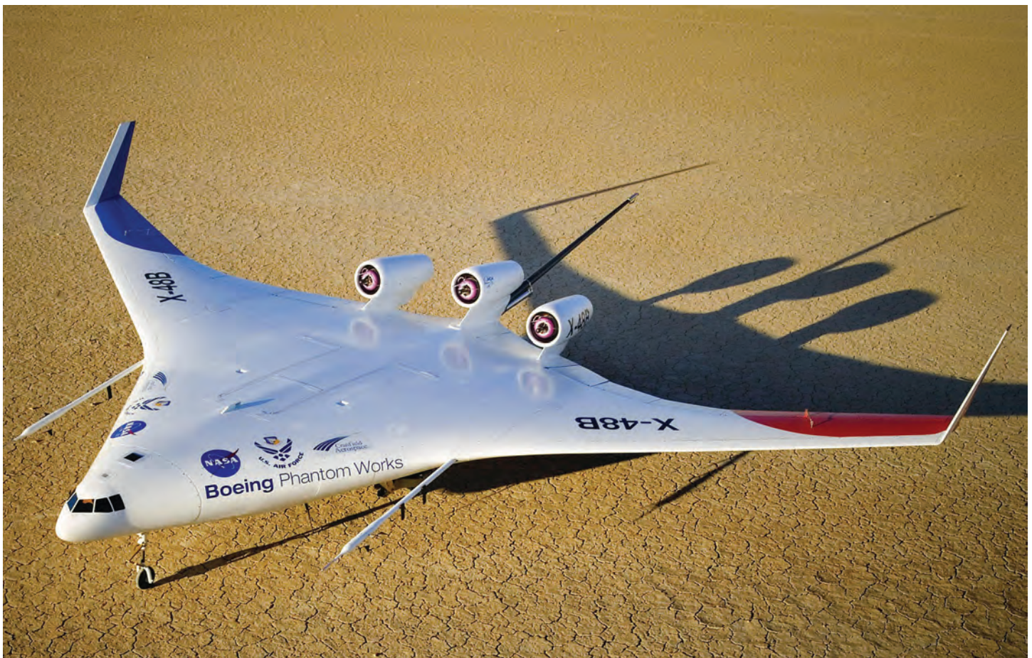
The Boeing-built X-48 Blended Wing Body demonstrator sits on Rogers Dry Lake near NASA’s Armstrong Flight Research Center. The 20-foot wingspan remotely piloted test vehicle flew for nearly six years, providing a valuable ground-to-flight database for controllability of the unique design through the flight environment.
