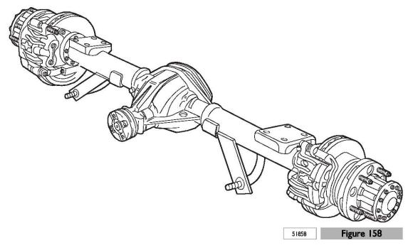
The wheel hubs are keyed, with "UNIT - BEARING" with "Long Life" lubrication, onto the arms of the axle casing. The bearings need no adjustment.
