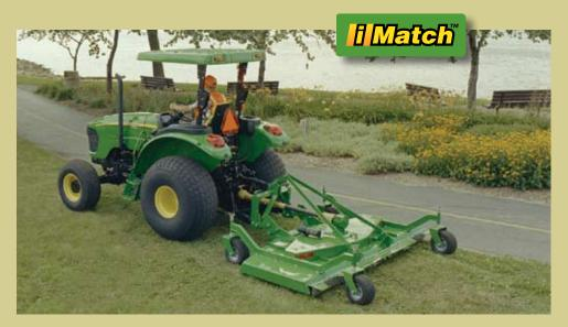
Frontier 20 and 21 Series grooming mowers can be fitted with the John Deere iMatch<sup>™</sup> quick-hitch system. iMatch converts your tractor's 3-point hitch to fixed hooks and attaching points for a super-quick connection. (iMatch hitch and implement A-frame kit sold separately.)
