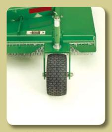
Stamped wheel yokes with air tires have spacers for quick and easy height adjustments.
