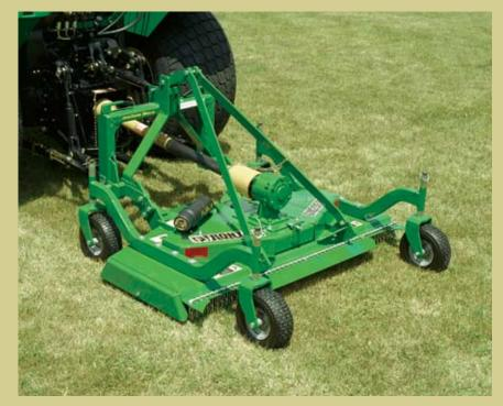
The standard-duty 20 Series is a rear-discharge, three-spindle mower. Each model can be front or rear mounted and is adjustable to cutting heights of 1 to 5 inches. A floating 3-point linkage (Category 1) and heavy-duty shielded PTO shaft make connections a breeze.
