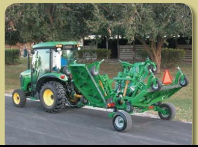
The 20 and 21 Series flex-wing grooming mowers feature heavyduty transport frames, high-flotation transport tires, and a single-action hydraulic folding wing system for easy transport and storage. SMV sign, transport safety chain and lights are standard.
