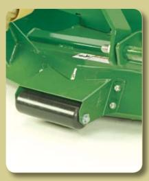
Standard anti-scalping rollers are mounted to the front of each cutting deck.
