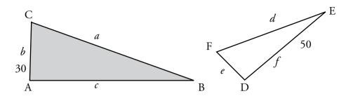
AB (side c) is 75 mm, AC (b) is 30 mm, DE (f) is 50 mm and angle B is 30°. What is the length of DF and how many degrees is angle F?
