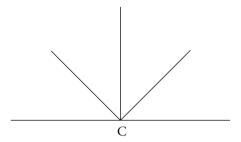
6 Construct angles of 60°, 30° and 15° at C. Check with a protractor.
