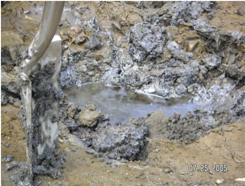
Figure 1. Silver colored sheen associated with PAH contamination from coal tar in the Cocheco River, Dover, NH.
