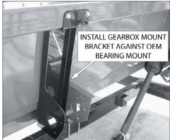
Figure 13, Gearbox mount bracket location
