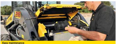
Maintenance and servicing on L200 Series skid steer loaders couldn't be easier, access for engine and hydraulic oil changes is via a removable cover on the left rear quarter. The ground level daily service points are grouped together at the rear for convenience.
