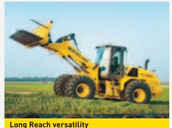
C Series wheel loaders offer Long Reach or Z-BAR configuration. Long Reach models offer a 0.4m increase in hinge pin height at maximum reach, ideal for loading trucks and high sided hoppers. These models are also up to 400kg heavier, so are well suited to forage ensiling.
