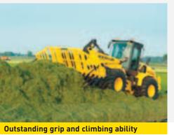
The front auto locking differential option provides 100% lock when required and the rear open differential ensures all the torque goes to where it's needed. The heavy duty rear axles, and rear axle oscillation of 24 degrees allows the C Series to cope with undulating terrain while maintaining traction and stability.
