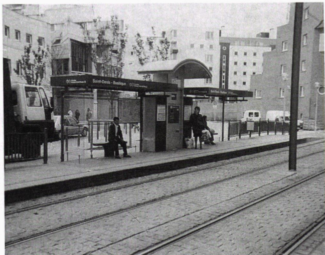
FIGURE 8 Low-level platforms are not as intrusive on a city street as are high-level platforms. This stop is in Paris.
