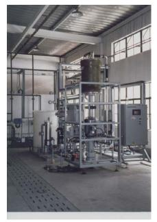
VSEP installed at a Volkswagen Plant for Coolant Recovery
