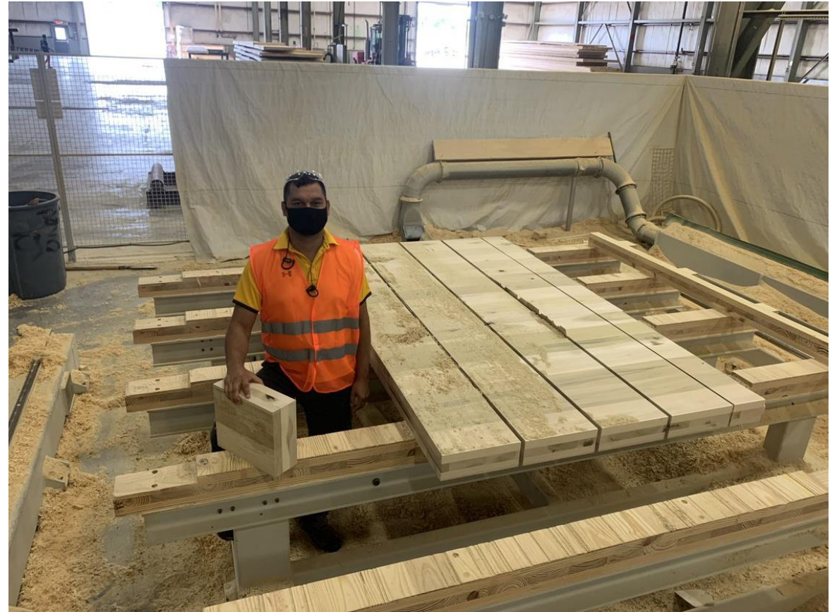
Yellow poplar CLT panels produced in Smartlam. Dothan, AL
