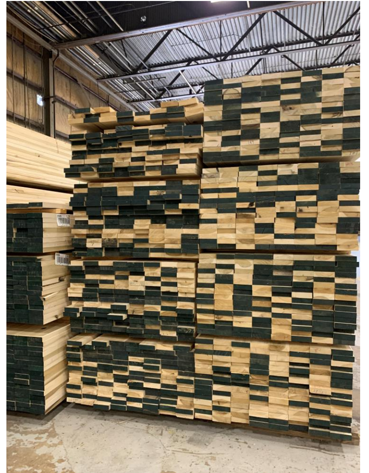
Structurally graded Yellow Poplar at Smartlam
