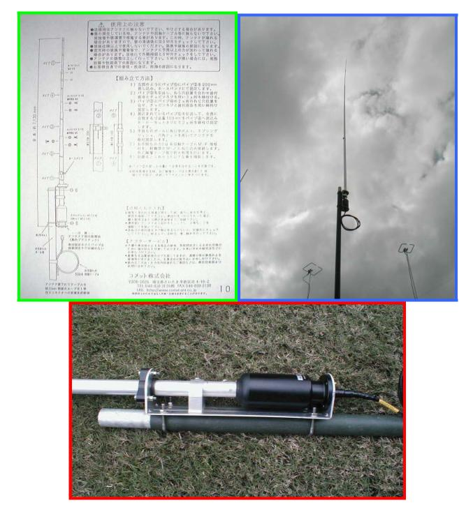
• The bottom picture shows the base of the antenna mounted to an aluminum mast section. Notice the exceptionally small matching network (black cylindrical section) of the antenna. No extended radials, this is it!
