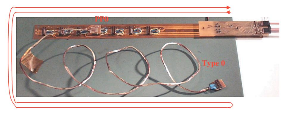
• data/clock from DORIC to VDC rerouted via PP0/Type 0 cables
