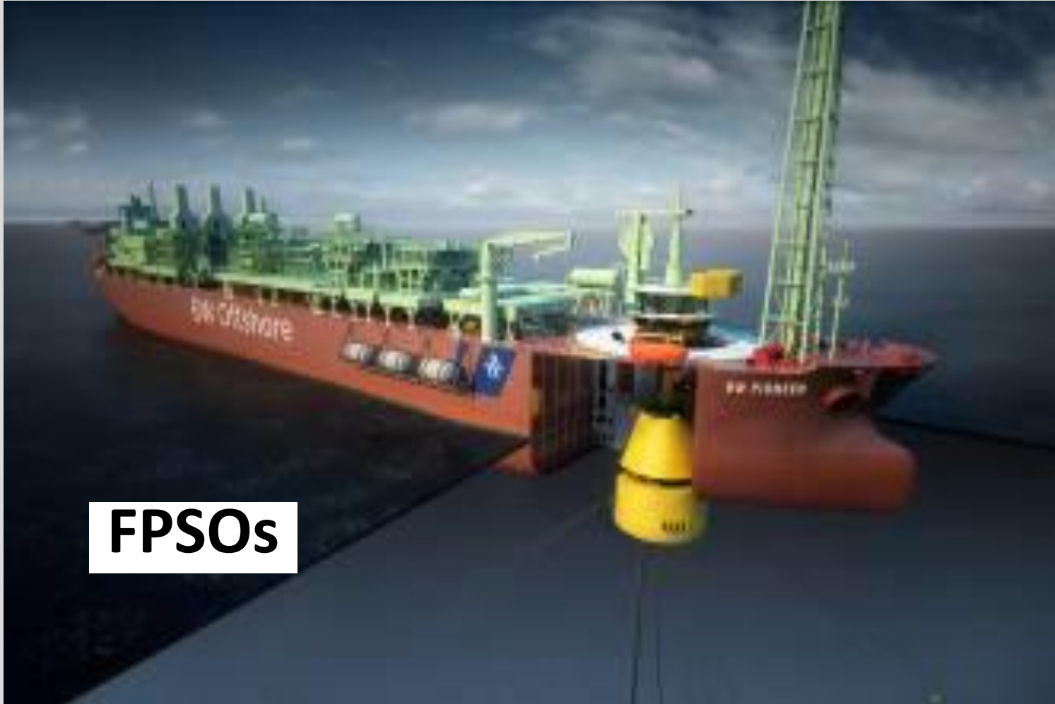
Petrobras FPSO BW Pioneer, with disconnectable turret, in 2,600m of water depth, in the Gulf of Mexico (Cascade and Chinook).
