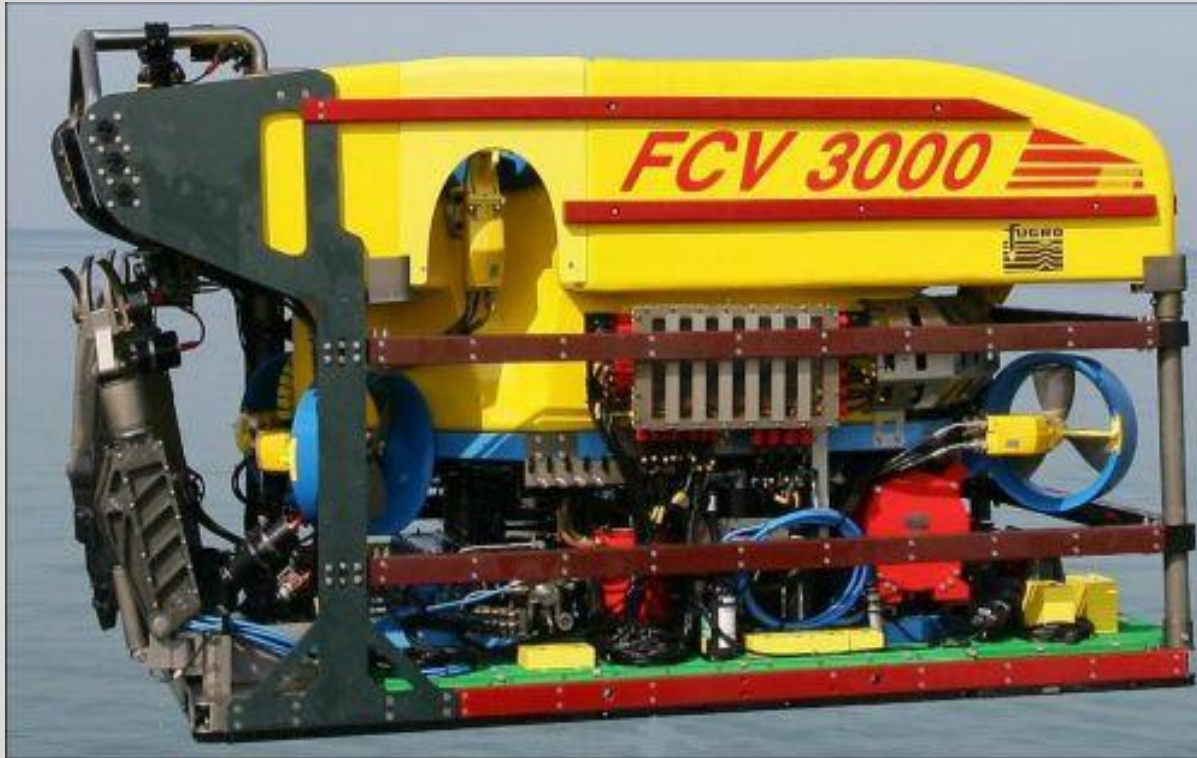
Typical heavy-duty, high-end ROV (Fugro)
