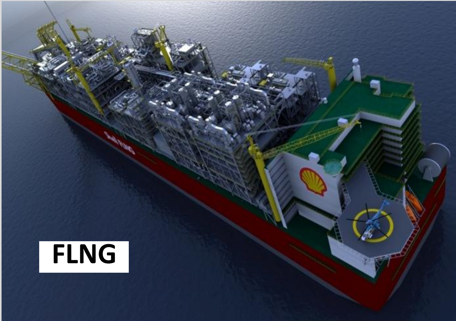
Prelude – Shell FLNG (488m, 600kt) to operate in Australia, to be built by Samsung, in Korea
