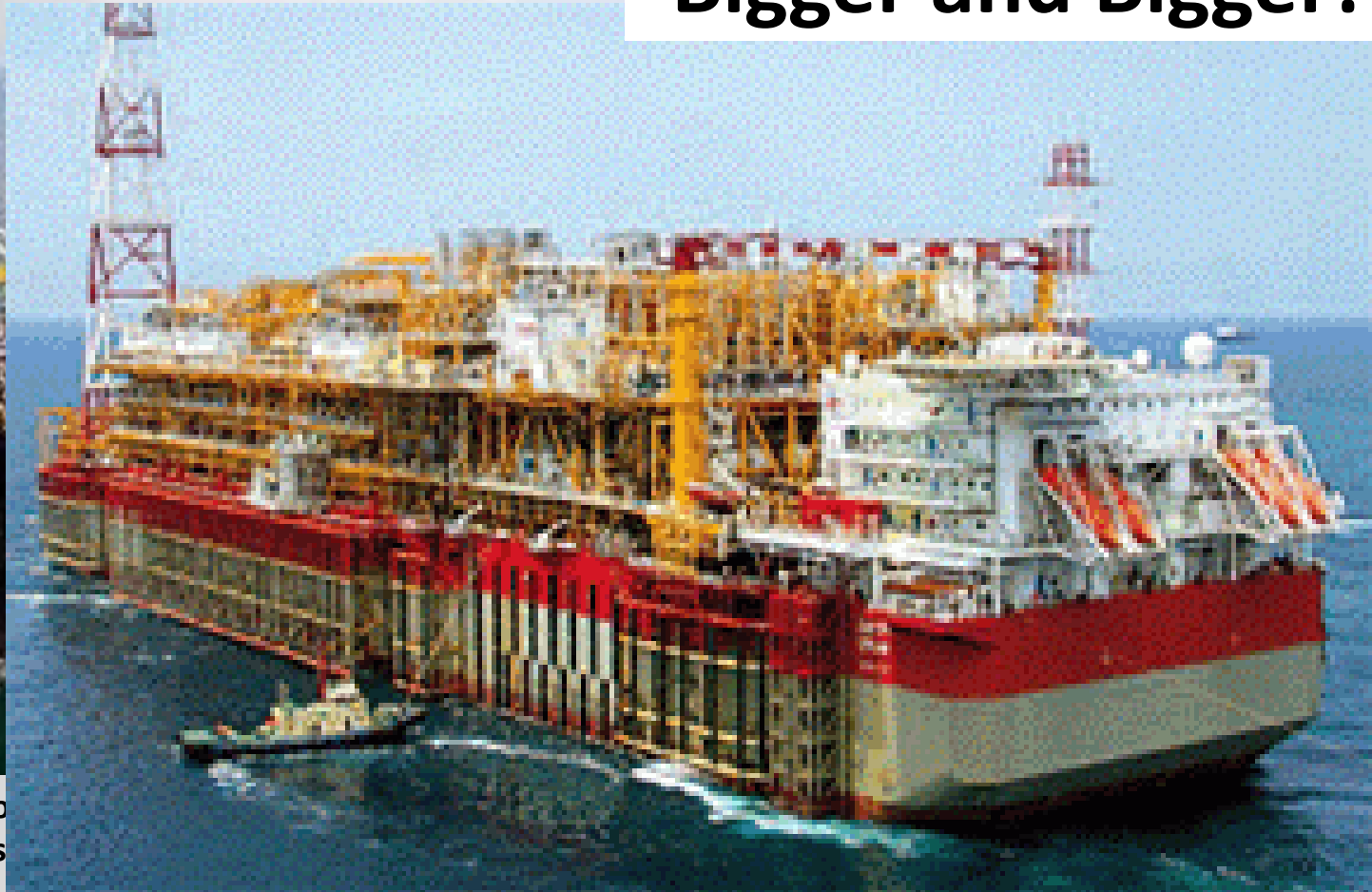
Usan FPSO, for Total in Nigeria - 320m long, 180,000 bpd production capacity, 2 million bbl storage capacity, to begin production in 2012 ( www.petroleumafrika.com ).
