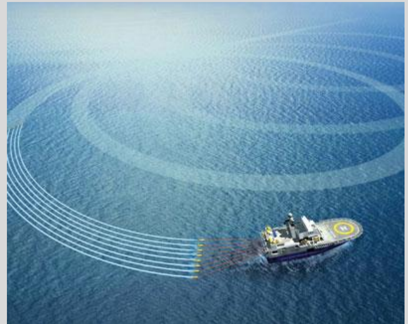
Coil shooting for full-azimuth seismic acquisition
