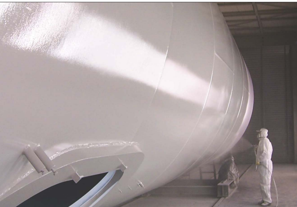
Direct-to metal polyaspartics can be formulated below 250 g/L and can give corrosion resistance in C3 environments similar to that of a combination of epoxy and polyurethane.
