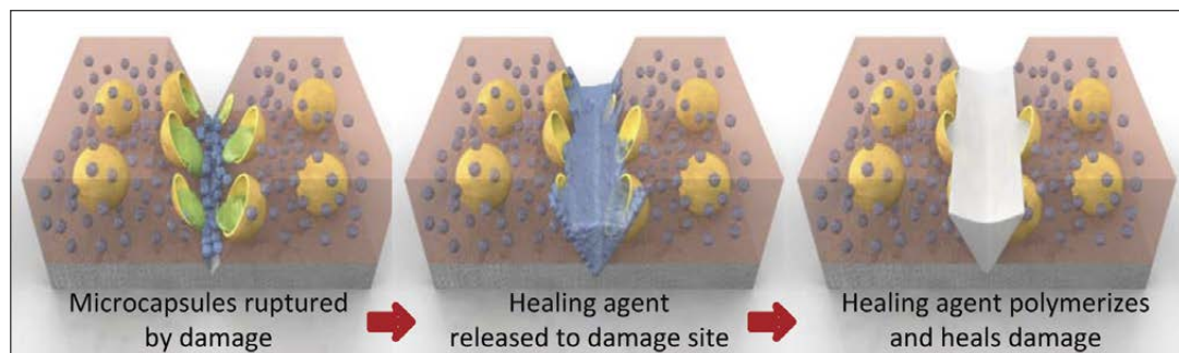
Fig. 1: Technical concept: Self-healing polymer coatings based on microencapsulation of healing agents.
