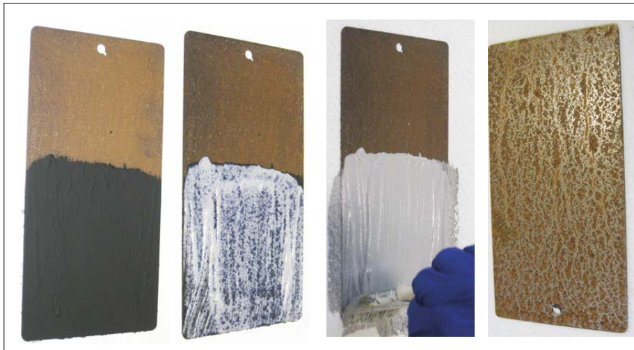
A new rust converter from Halox converts rust into a paintable protective black layer that seals out moisture and protects against corrosion. Courtesy of Halox
