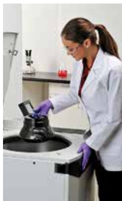
1. Place rotor into the centrifuge chamber
