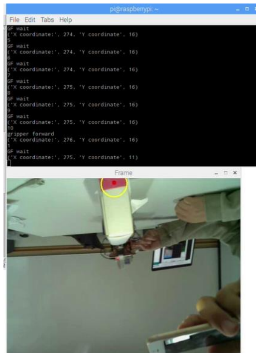
Figure 3-5: Results shown on Raspberry pi when robot move forward after grip
