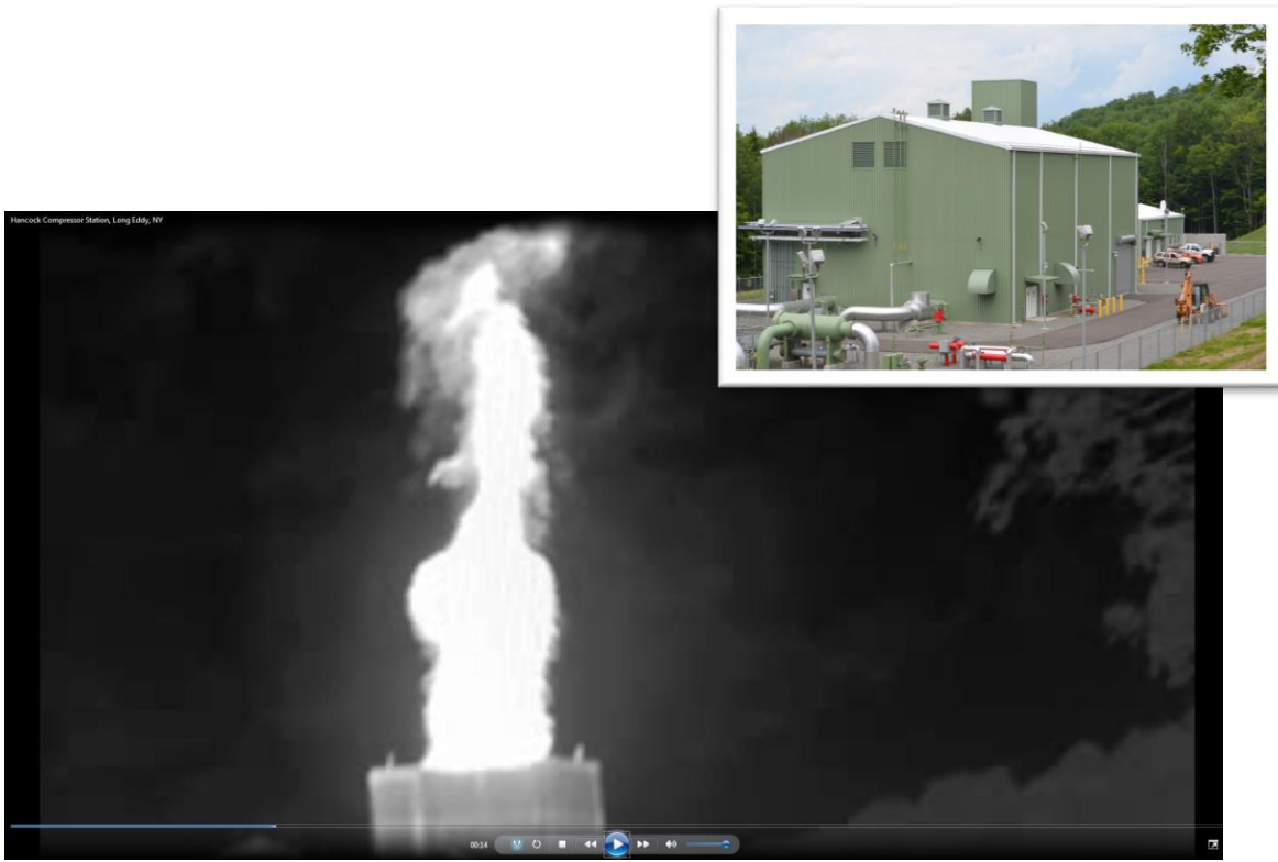
Emissions seen with optical gas imaging, Hancock Compressor Station, Sullivan County, New York. Images by Earthworks.
